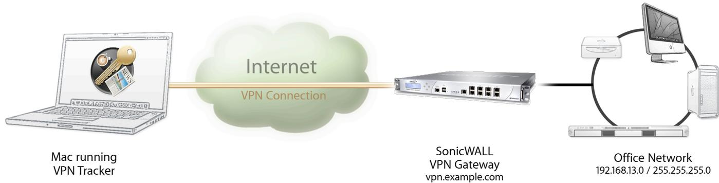
This guide assumes that the Mac running VPN Tracker already has internet connectivity. The office's SonicWALL (the "VPN Gateway") is also already connected to the Internet and can be accessed through a static IP address or DNS host name. In our example setup, we will be using a host name: `vpn.example.com`.
