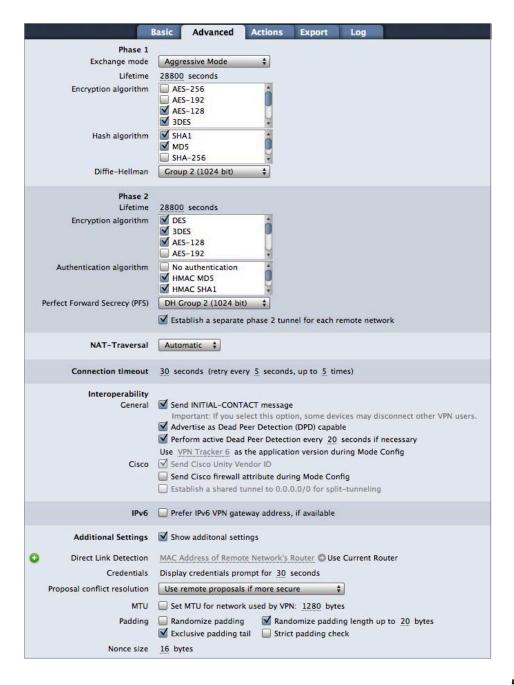
An IPsec VPN connection is established in two phases. In each phase, VPN Tracker sends the algorithms it is willing to use, as well as a few other settings to the VPN gateway. The VPN gateway then selects one set of algorithms ("proposal"), or responds with an error if it does not agree to use any of the proposed algorithms.
